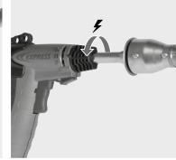
Open the flow wheel to the maximum by turning in the direction of the + arrow and check the the lance is in the operating « position lightening bolt ».
